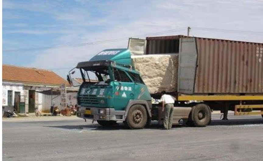
FIGURE 2: A TRUCK IS TRANSPORTING A HUGE STONE. WHILE THE TRUCK IS IN MOTION, THE STONE IS ALSO IN MOTION. A DEER SUDDENLY JUMPS INTO THE ROAD AND THE DRIVER SLAMS THE BREAKS. THE TRUCK STOPS BUT THE STONE MOVES FORWARD BECAUSE THE STONE, THAT IS IN MOTION, FIGHTS TO STAY IN MOTION. RETRIEVED FROM HTTPS://WWW.EXPII.COM/T/MASS-AND-INERTIA-632
