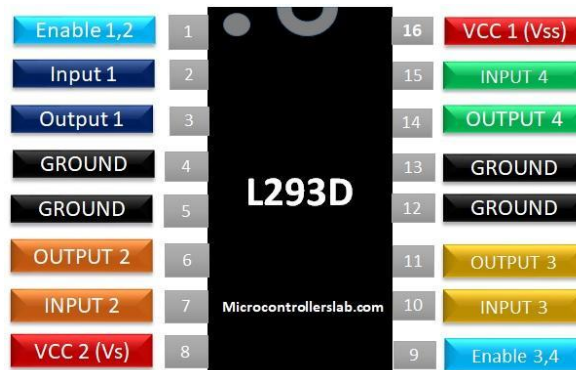
Image 11: Pin details of the L293D control chip. Pin 1: sense On/Off motor #1; Pin 2: input for the direction of the motor #1 spinning; Pin 3: output of motor #1; Pin 4-5: ground; Pin 6: output of motor #1; Pin 7: input for the direction of the motor #1 spinning; Pin 8: voltage pin for the motors. It should be comprised between 4,5V and 36V; Pin 9: sense On/Off motor #2; Pin 10: input from the GPIO for the direction of the motor #2 spinning; Pin 11: output of motor #2; Pin 12-13: ground; Pin 14: output of motor #2; Pin 15: input from the GPIO for the direction of the motor #2 spinning; Pin 16: chip power. The tension should be comprised between 4,5V and 7V (image from: https://microcontrollerslab.com/l293d-motor-driver-ic-introduction-pinouts-example/ )
