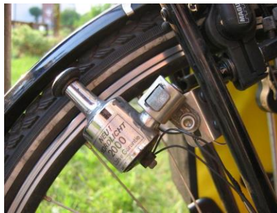
IMAGE 6: BOTTLE DYNAMO MOUNTED ON A BICYCLE. (IMAGE
