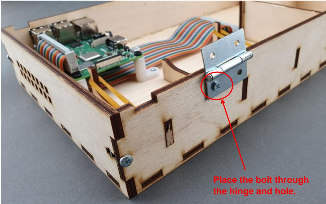
Place the bolt through the hinge and hole.
