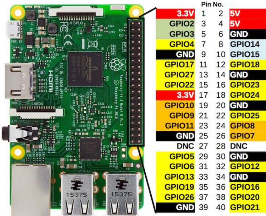
FIGURE 6 RASPBERRY PI GPIO AND PIN ASSIGNMENT
