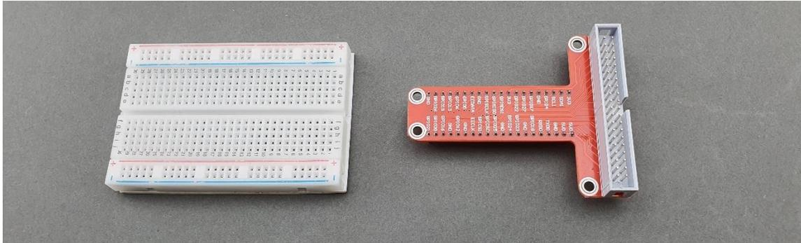
**Make sure the 40P T-Cobbler covers both sides of the breadboard and then press it against the breadboard.**
