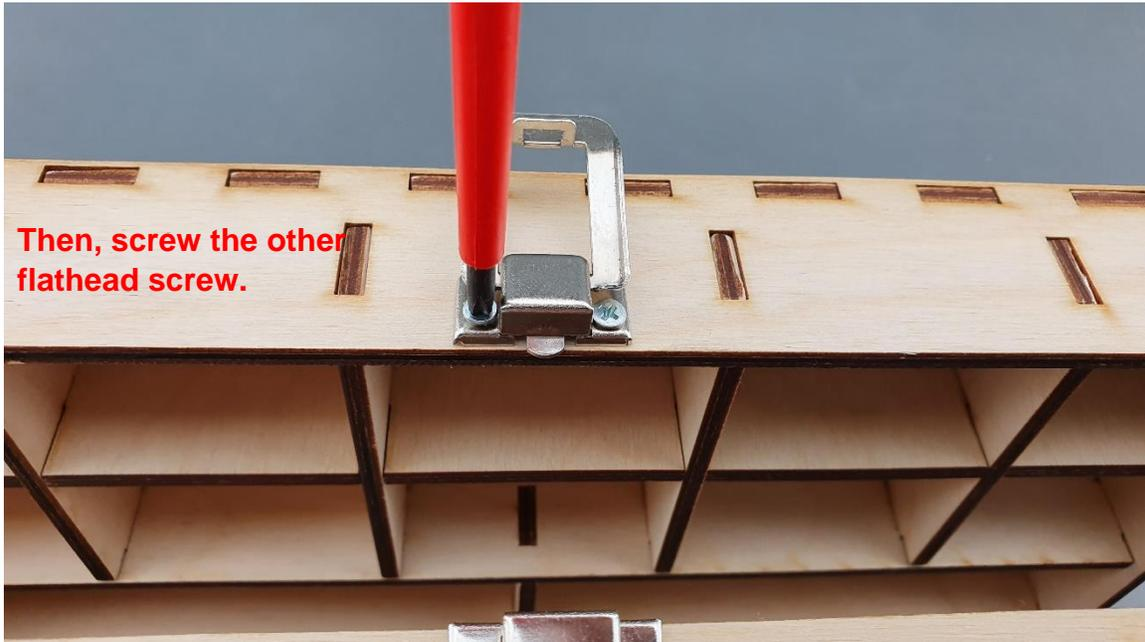
**Step 4 – Make sure the two lock pieces are aligned and the lock is working:**
