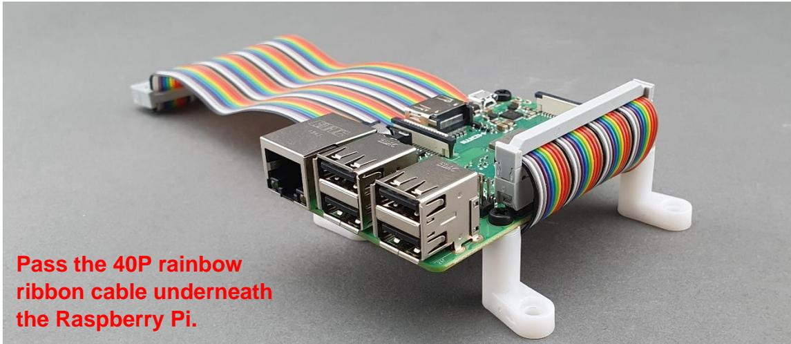
**Step 4 – Mount the Raspberry Pi to the lower-case:**
