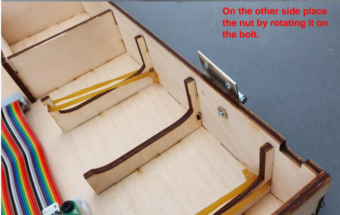
On the other side place the nut by rotating it on the bolt.
