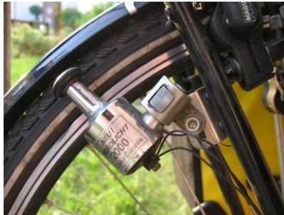
IMAGEM 6: DÍNAMO GARRAFA INSTALADO NUMA BICICLETA (IMAGEM RETIRADA DE:
